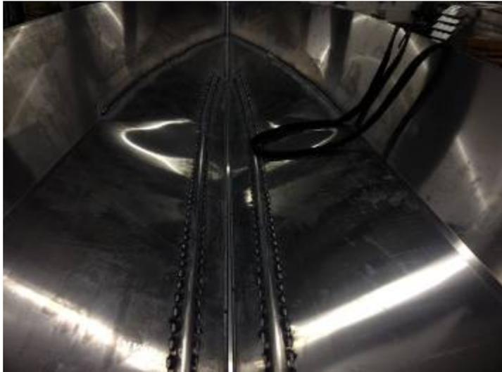
Starweld hulls are two piece hull w/ sides attached to each piece. They are assembled by welding each half of the hull / side combo piece of .100 gauge into a full length extrusion and then welded from the inside to give a clean look on the hull and add superior strength from within accompanied with the TBC – (Torsion Beam Construction) stringer system.
