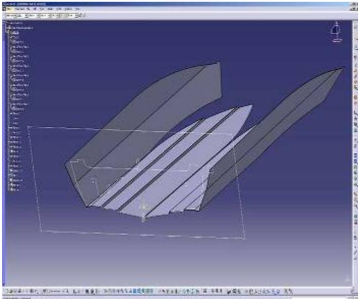
Tracker uses a two piece hull and two side for a total of 4 pieces which are then place into an extrusion and welded plus the transom which requires much more welding to make the hull complete. This creates more opportunities for weakness and inconsistency throughout the hull. The finish is sub –par when you look at there boat and welds compare to a Starweld.
