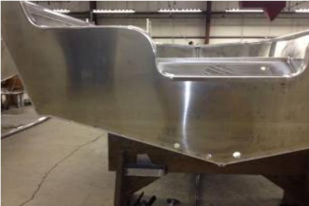
Starweld has a 17 degree deadrise at transom for a very stable platform at the aft section of the boat with less degree of listing when weight is in one corner. We also have a full length reverse chine which runs from the stern to the bow of the boat that directs water down and away from the boat for quicker planing, improved cornering and a smoother, drier ride overall.
