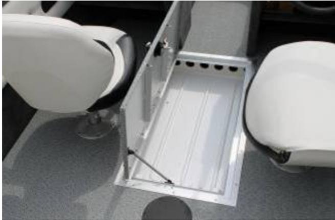
Starweld has lockable in floor rod storage for 6 –rod combos up to 8'in length plus has port and starboard side rod storage as well. Side storage makes for a much stronger gunnel and plenty of room to mount track, rodholders and downriggers.
