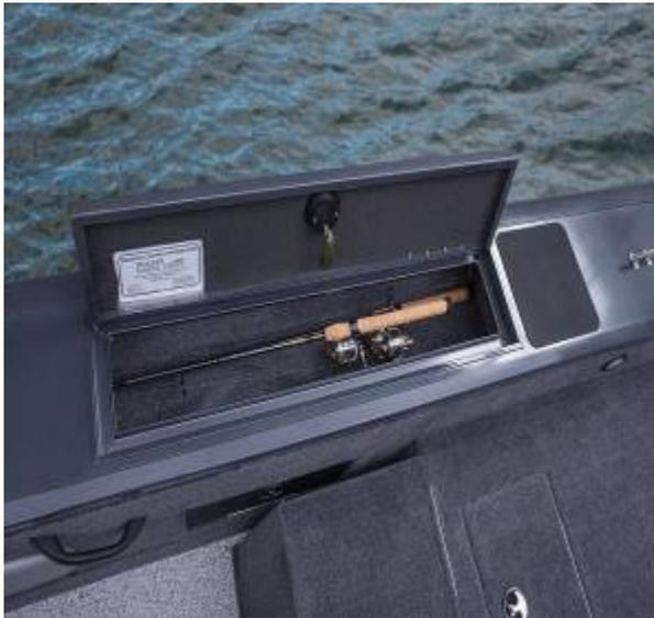
Tracker has an open in floor compartment which can hold rods but is not dedicated to rods therefore making it a sloppy storage system. They have top load rod storage on each side but again very poor storage supports. Plus tough to mount track, rod holders and downriggers due to door.
