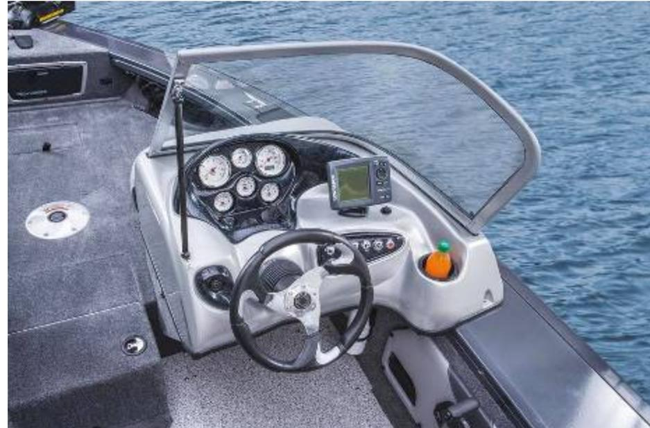
**TRACKER** – Glossy plastic grey console which is less appealing to the eye. Integrated drink holder. Includes speedometer, tachometer, voltmeter, fuel gauge, AM-FM/CD stereo w/MP3 jack and tilt hydraulic steering as standard features.
