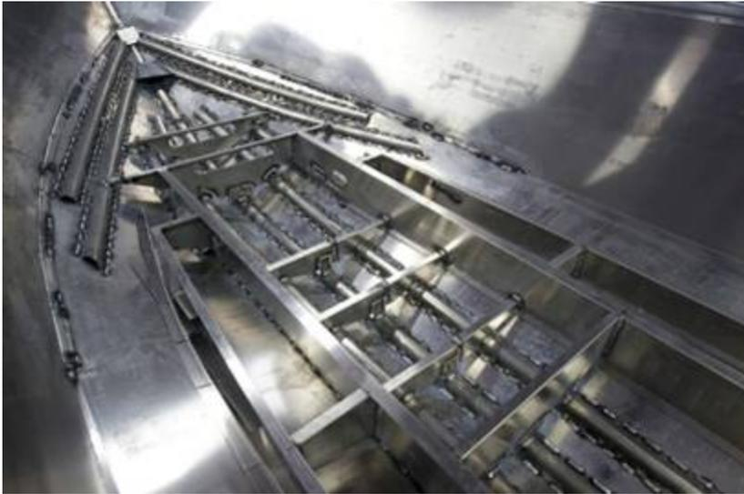
Starweld Torsion Beam Construction is superior to our competition for durability and strength. Instead of flat I-Beams you find on many boats Starweld uses the exclusive Starweld Torsion Beam Construction (TBC) Stringer system for exceptional strength and durability against shock absorption from waves. This bow is also considerably stronger due to our unique heavy duty machine formed ribs.
